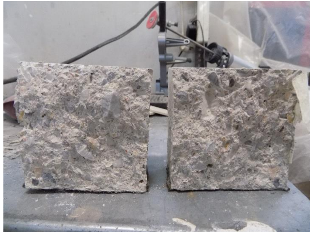
Fig.4 Split specimen with zero water penetration
