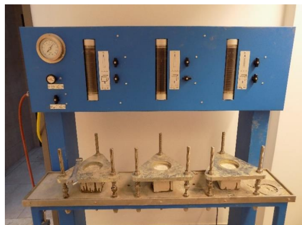
Fig.2 Water penetration testing setup
